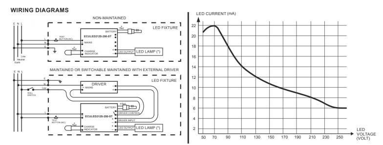
(\*)LED LAMP: Min 30V, max 250V, (Serial connected LED group or LED PCB - Ref to figure) Ballast Lumen Factor (BLF)=Emergency Ballast Lumen Factor (EBLF): % Lumen output emergency mode/mains mode .EBLF of different lamps/luminaires could be calculated easily as following:
